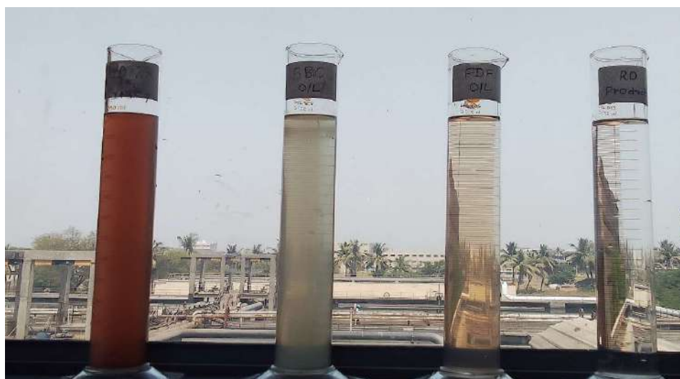
Figure 3.5 Stage wise effluent quality – Colour, TSS and Turbidity, a) Raw influent b) O/L Primary Treatment c) Outlet Secondary d) RO permeate – Recycle water
